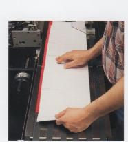
A Single-handedly unload 10,000 tabs/hour. At 10,000 tabs per hour, how can one operator keep up? Indexes collect in an overlapped or "fanned" position on a slowly moving, conveyor. The conveyor holds up to six minutes of the machine's production. One person can easily handle the entire operation.
